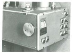
AUTOMATIC CYCLE CONTROL Adjustable dials control limit switches for operating spindle traverse motor and electric feed clutch on adjustable spindle head.
